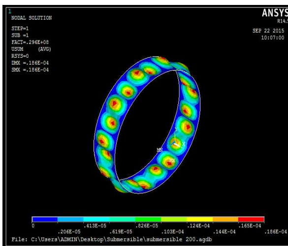
Figure 19: Buckling Mode and Circumferential Wave Pattern of 1 st Buckling Mode (n=11)
